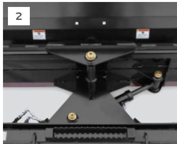
1. 4° SIDE-TO-SIDE OSCILLATION FOLLOWS UNEVEN SURFACES
